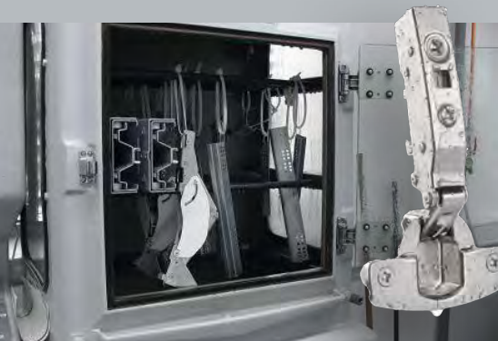
Condensation water test
